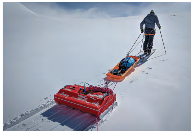
Toby Harper-Merrett pulls a 100 megahertz ground-penetrating radar system in a grid pattern between Prospector's and Russell peaks. Photo: Zac Robinson, courtesy of the Royal Canadian Geographical Society
