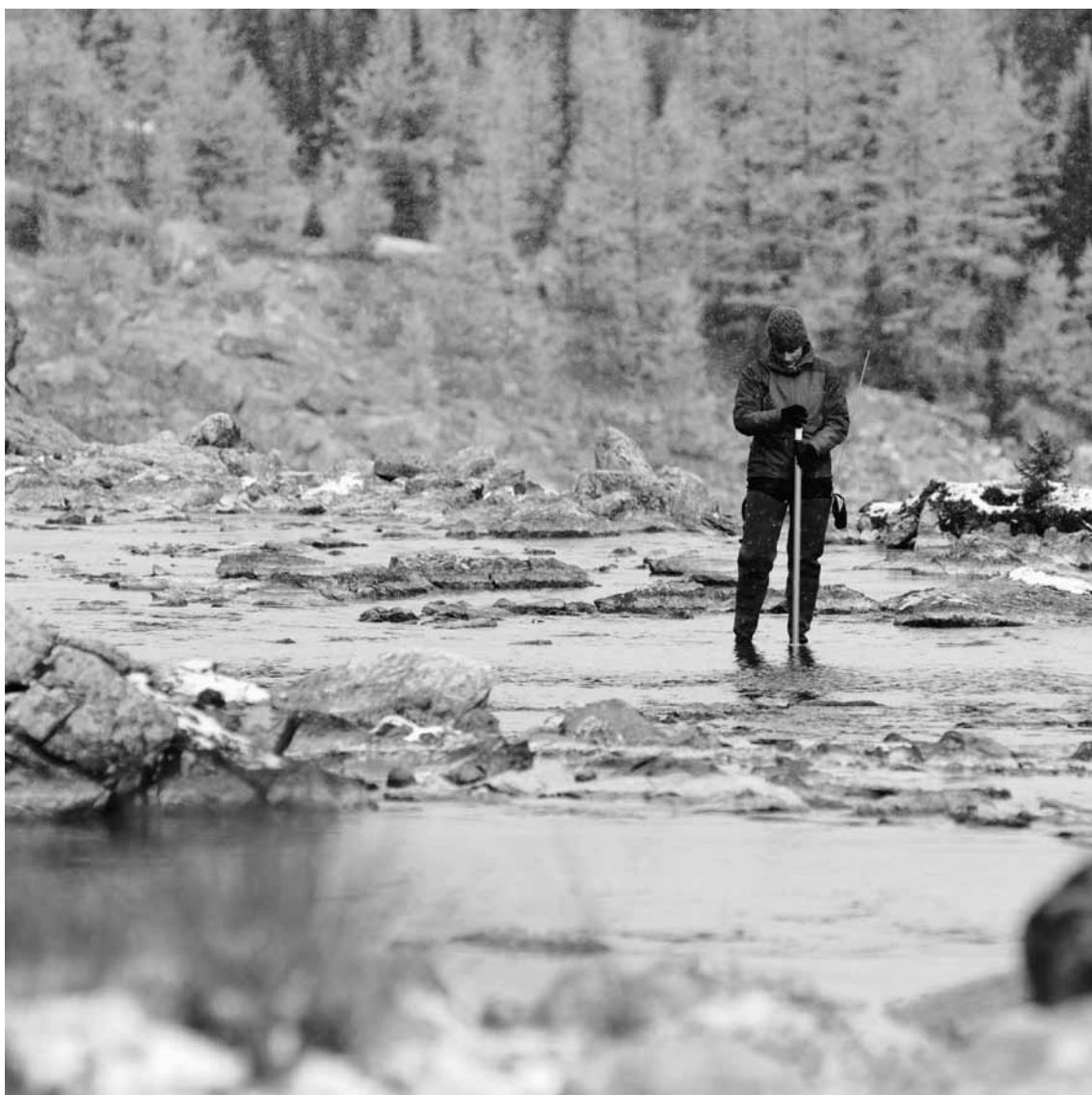
Jackie Randall takes advantage of one of the last days of the fall season for stream flow gauging on Upper Opabin Creek. Photo: Andrew Querner
