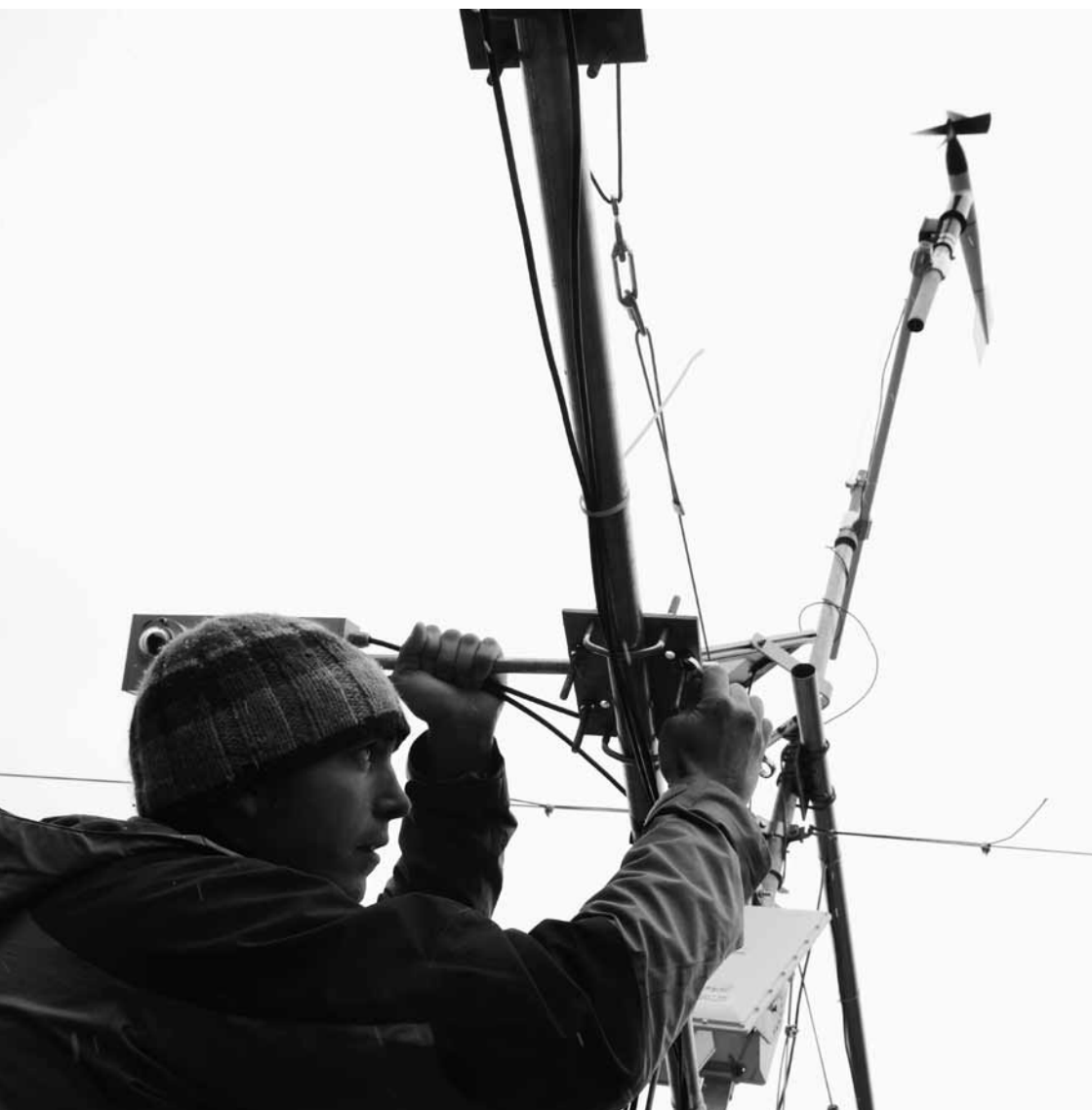
Greg Langston secures the instrumentation on the Opabin meteorological station to ensure it survives another winter season. Photo: Andrew Querner
