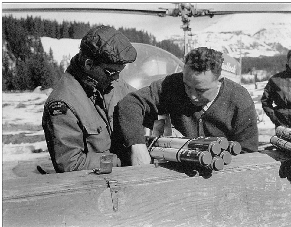
Heli-bombing. Helicopters were also employed to trigger avalanches that threatened major highways. In this photograph, Peter Fuhrmann and Andy Anderson are making a 10 lb. bomb out of nitro canisters. This substance was considered a blasting agent and was therefore exempt from regulations prohibiting carrying high explosives in helicopters. Photograph courtesy of Parks Canada.
